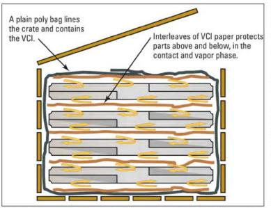
To protect large metal stampings from corrosion during shipment and storage, the stamper lines the crate with a low-density polyethylene bag impregnated with VCIs that protect the parts that contact the bag as well as parts in proximity to the bag. Interleaves or paper or film VCI sheets may be added, laid at intervals as the parts are stacked to ensure delivery of enough VCI to protect parts in the center of the crate.
