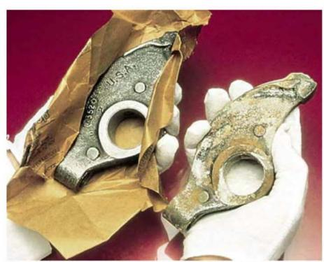
VCI molecules align on metallic surfaces to a depth of three to five molecules, migrating into recesses on parts. The layer of molecules passivates the charged surface and creates a barrier that prevents corrosion-causing materials such as moisture, salt, dirt and oxygen from depositing directly on the parts.
